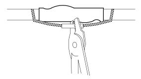
If necessary, cut excess length from braid straps. Crimp the braid straps together into an uninsulated splice connector, then secure the connector at the indented area with one and a half wraps of electricians' tape.
