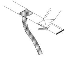
**WARNING:** DO NOT CUT BUS WIRES
