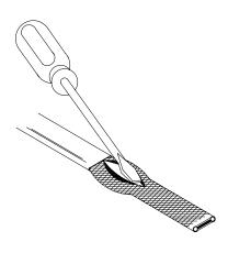
**5** At the bulge, separate the braid to make an opening.
